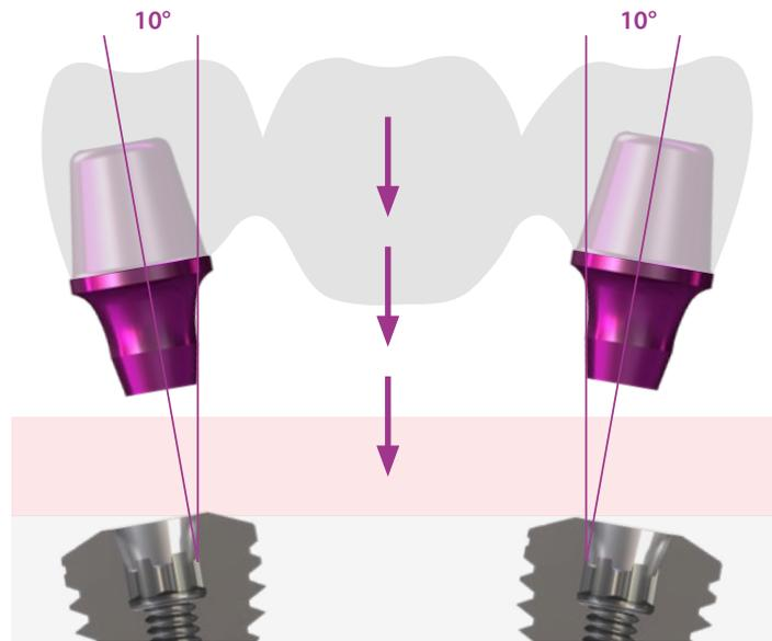
The construction can be easily integrated and occlusally screwed. The long cone directs the lateral and occlusal forces onto the implant directly and therefore protects the screw against loosening and breakage.
