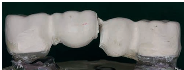
Fig. 33: Fracture of a BioHPP bridge produced by CAD/CAM. 43)
