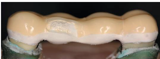
Fig. 39: Bridge after load test with chipped veneer. 52)
