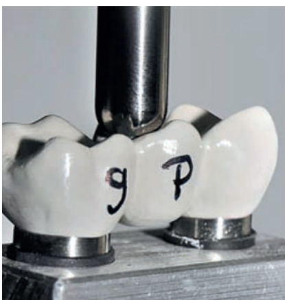
Fig. 19: BioHPP bridge during the test. 24)
